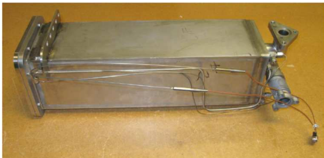
hot reformat desulfurizer
